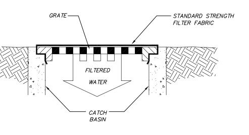
NOTE: ONLY TO BE USED WHERE PONDING OF WATER ABOVE THE CATCH BASIN WILL NOT CAUSE TRAFFIC PROBLEMS AND WHERE OVERFLOW WILL NOR RESULT IN EROSION OF SLOPES.
