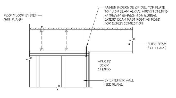
GO FLUSH HDR CONNECTION @ ROOF SCALE: 3/4"=1'-0"
